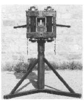
The euthytonon was invented in mid-fourth century BC. The weapon is powered by two torsion spings consisting of rope bundles. On each end of a torsion spring there is a bronze washer (*modiolus*) holding an iron lever (*episygis*). The two torsion springs and the four modioli are clearly visible in the reconstruction displayed here, also the two arms of the weapon coming out at the sides.
